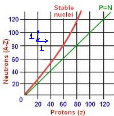
Nuclei that are above the stability band have too many neutrons & are beta emitters (changing a neutron into a proton)
